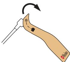
2. Attach new tape in same direction as used tape
