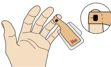
3. Squeeze top and bottom of finger to secure tape.
